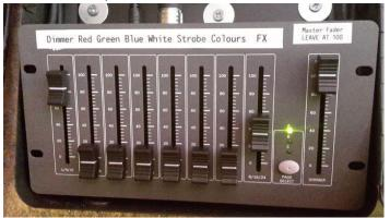
10 DIMMER can be adjusted to give the desired brightness.
